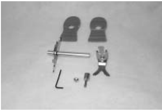
C. Place the plastic (polypropylene or copolymer) and metal components in 400° oven until the plastic clears. Then place PolyCar-C™ into the oven for 2-3 minutes, or until pliable.
