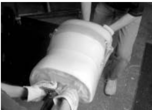
G. Immediately vacuum form the last piece of copolymer over the entire model.
