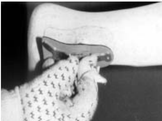
E. Immediately place the heated ankle joint (the PolyCar-C™ assembly) on the cast where it is outlined.
