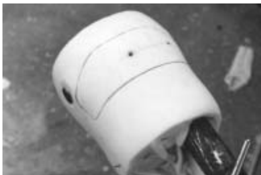
A. With RGO hip joint hardware in place, lay out pattern for unidirectional PolyCar-C™ reinforcement.
