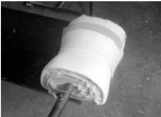
E. To evacuate all air between the first and second layer of copolymer, place a covering of fish net on top of the first piece of copolymer.
