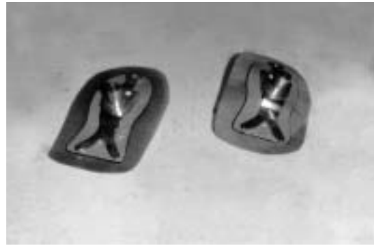
D. After heating to approximately 400° F, place the PolyCar-C™ on the ankle joint assembly and replace in oven for 1-2 minutes.
