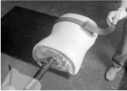
C. Position heated PolyCar-C™ and backup 1/8" copolymer piece on the model and peel away the Teflon backing.
