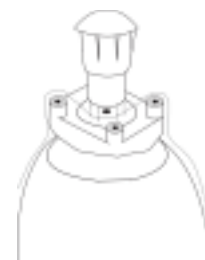
Following thermoforming, Use A Hole Punch To Cut Out A Plug of Plastic Over the 5/16" Center Screw F
