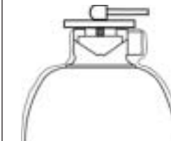
Slide Heated Flattening Plate On Set Screw. attach Cam Lock and Rotate To Compress Plastic Against 4-Hole Posts
