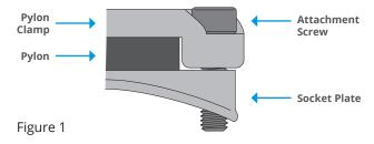
Before attaching the socket plate to the posterior socket wall, ensure that the longest screw in the kit is installed and the foot is place between the pylon clamp and socket plate as shown in Figure 1. The screw will, in most cases, protrude through the socket plate. Adding silicone spray to the screw end can simplify removal.
