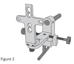
3. Attach the Adjustable Alignment Bracket to the Transfer Fixture by placing two M6 socket head screws through the slots in the Transfer fixture into the threaded holes 5 & 6 (Figure 4) in the Adjustable Alignment Bracket and tighten to prevent movement.
