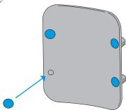
3. Apply a liberal amount of Fabtech +PLUSeries® 60 Second Adhesive to the rear surface of the Socket Plate and press onto the socket at the determined mounting location. Hold in place until adhesive has cured.
