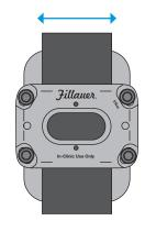
Once final alignment is found, the foot can be mounted to the socket with the Fillauer Posterior Mounting Bracket Kit (180-10-3000) or directly laminated onto the socket.
