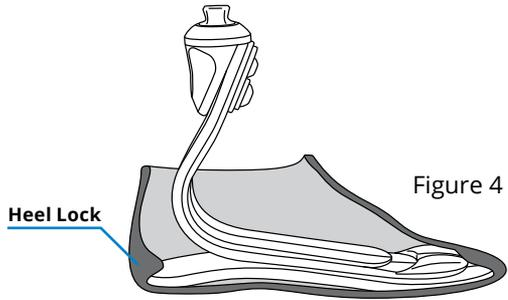
**IMPORTANT: The heel of the lower foot plate must slide into the heel lock in the foot shell for proper alignment and to secure the foot in the foot shell (Figure 4).**
