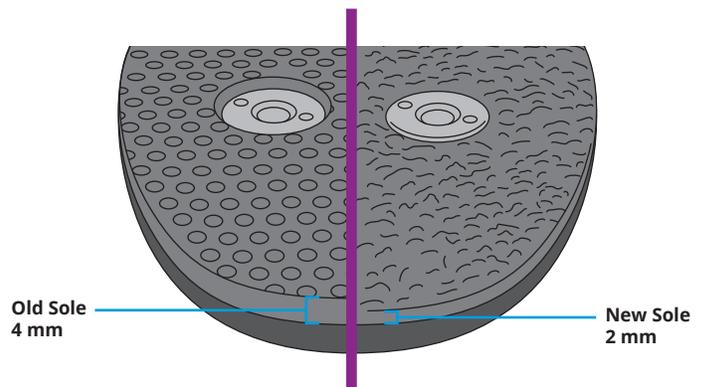
2. If the correct sole was used, then proceed to **ProCover Installation**. Otherwise, replace the old soling using the instructions provided with the replacement soling sheet.
