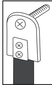
6. Spray a generous amount of silicone spray (PN-199026) on the upper upright. Slide forming/contouring sleeve over upright until it meets the joint.
