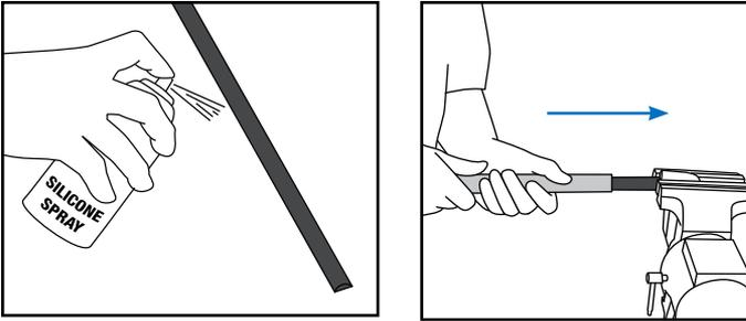
*Note: When applying forming/contouring sleeve, push the sleeve on by applying pressure to the sleeve at the proximal end of the upright. When removing sleeve, pull the sleeve off by applying pressure to the sleeve at the distal end of the upright.*
