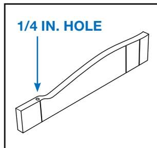
3. Contour calf band using conventional methods. Make sure that the calf band attachment areas are parallel to the upright positions. Bend stirrup into position and insure that ankle joint axis is square to the longitudinal axis.
