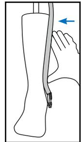
*Note: A 1/8 in. spacer should be used at ankle joint location to account for contouring sleeve thickness during contouring process.*
