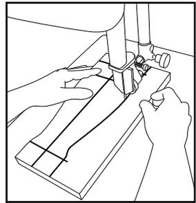
3. Contour calf band using conventional methods. Make sure that the calf band attachment areas are parallel to the upright positions. Bend stirrup into position and insure that ankle joint axis is square to the longitudinal axis.
