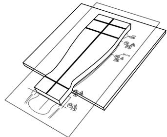
5. Mark attachment hole position using the ankle joint or drilling template. Drill attachment holes using a drill bit that corresponds to the correct attachment screw. Position TFC upright into joint attachment notch of the ankle joint. Using screws attach flattening plate over upright and secure them firmly.
