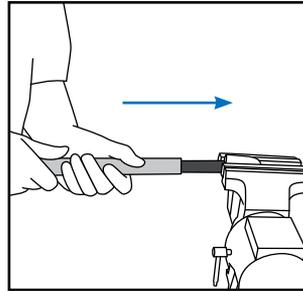
*Note: When applying forming/contouring sleeve, push the sleeve on by applying pressure to the sleeve at the proximal end of the upright. When removing sleeve, pull the sleeve off by applying pressure to the sleeve at the distal end of the upright.*
