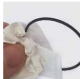
Cleaning and inspecting O-ring.
