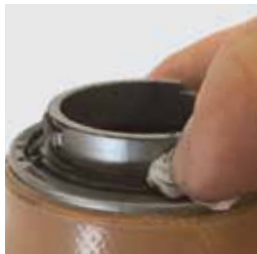
Cleaning Lamination Ring.
