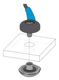
If possible, install the sensing electrodes between 1 and 2 inches (25 – 50 mm) apart. This may not be possible with extremely short transradial fittings. In those cases, make sure the electrodes are not touching. The ground electrode (black lead) can go anywhere in the socket with good electrode contact, at least one inch from sensing electrodes if possible.
